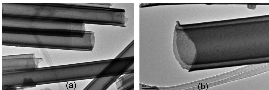
TEM view of resultant coaxial \text{HfO}_2 nanotubes following release from the AAO template and removing the sacrificial spacer \text{Al}_2\text{O}_3 layer
